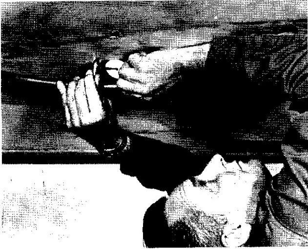
STEP 7 — Insert J-bolt, twist ¼ turn — hook over cutout in crossmember (see section A-A). Hold down on threaded end insert plastic retainer snug against trailer.
